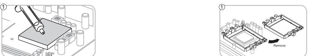
Remove the original retention frame from the motherboard.
