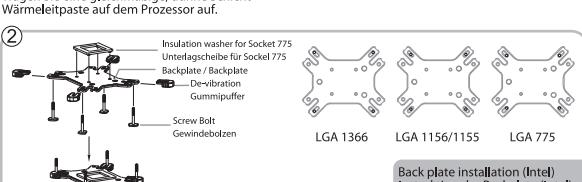
As illustrated, fix the insulating washer,De-vibration buckle and screw bolt to the mounting holes of back plate.
