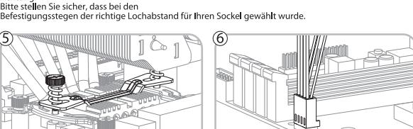
Place the heatsink onto the processor, attach the retention plate to the mounting bracket (INTEL) and fasten the screw bolt into corresponding holes by hand or tools, and secure it with a nut.
