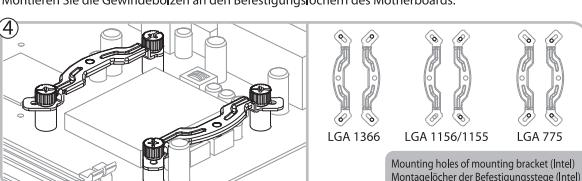
Assemble the insulation pillar into double-screw bolt; Place the screw bolt at the right places according to the holes of mounting bracket (INTEL), then fasten by nuts like shown.
