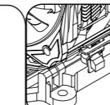
(E) As illustrated, put the heatsink onto the processor and hook the vertical clip onto the retention frame tab.
