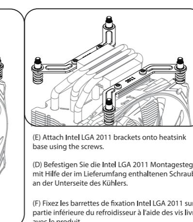
(E) Attach Intel LGA 2011 brackets onto heatsink base using the screws.
