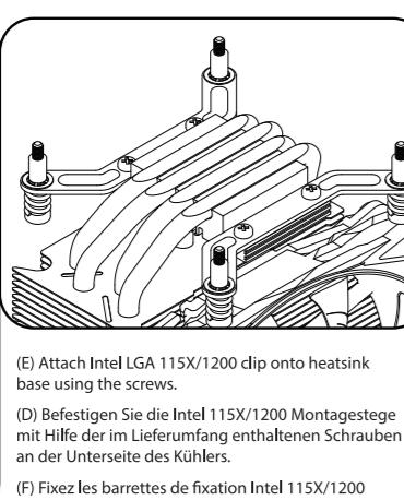
(E) Attach Intel LGA 115X/1200 clip onto heatsink base using the screws.
