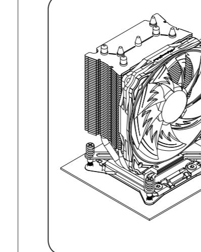
(E) Put the cooler on the processor, check your socket type and ensure all screws through the motherboard mounting holes. Position the clip as shown in the picture and then push down to secure the cooler.
