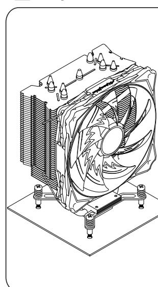
(E) Put the cooler on the processor, check your socket type and ensure all screws through the motherboard mounting holes. Position the clip as shown in the picture and then push down to secure the cooler.
