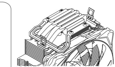
(E) Attach the AMD metal clips onto heatsink base using the screws.
