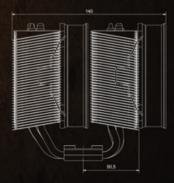
To make sure that the ATLAS fit in your case please measure the distance from the top panel. If this distance is bigger than the height of the cooler + 30mm it should be no problem to install the ATLAS.
